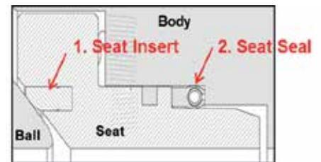
Figure 3: TMBV Single Piston Effect seat design, Saint-Gobain Cryogenic Test Rig
