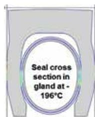
Seal designs were evaluated based on the evolution of interaction between sealing force and contact length with the hardware.
